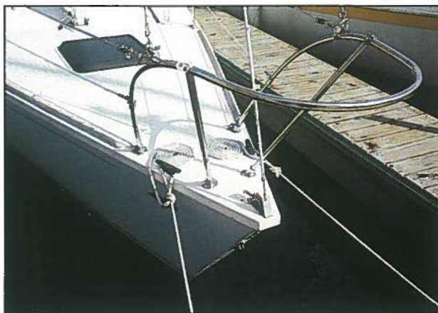
The foredeck should provide a secure pulpit, strong stanchions and lifelines, and a toe rail to brace against. Cleats on a boat not equipped with a samson post must be strong enough for anchoring and for any towing. Fittings on this racing sailboat have been chosen for their light weight and not their strength.
