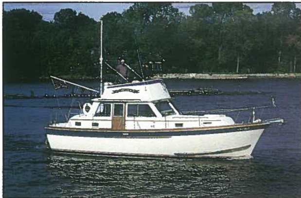
The trawler was originally designed as a low-speed, seaworthy fishing vessel. As a recreational type, trawlers are fuel-efficient and offer many on-board living advantages.
