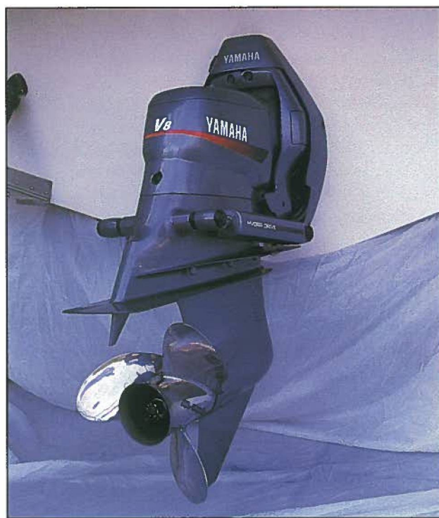
An inboard-outboard’s “outdrive” or “lower unit” permits the coupling of a powerful inboard engine with a steerable and trimmable propeller shaft. This configuration has become popular for powerboats from 18 to 28 feet (5.5 to 17.7 m).
