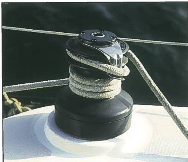
A winch revolves in only one direction, resisting the strain of sheets and providing extra power for trimming sails. Self-tailing winches like this one allow one person to do the work of two.
