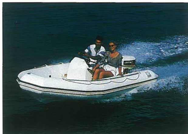
Rigid-hull inflatable boats, often called RIBs, are constructed both as small tenders and as larger sportboats. They combine the benefits of a conventional hull with inflatable flotation and stability.
