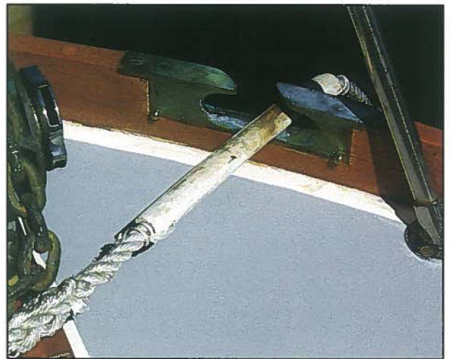
Chafe guards should be used on any lines that pass over an abrasive surface. They may be a purchased item, as above, but can be home-made by using slit garden hose or special tape.
