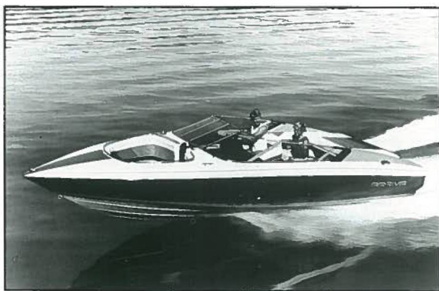
Hydrodynamic force lifts a planing hull partially out of the water, reducing drag and wave-making resistance. This makes high speeds possible.
