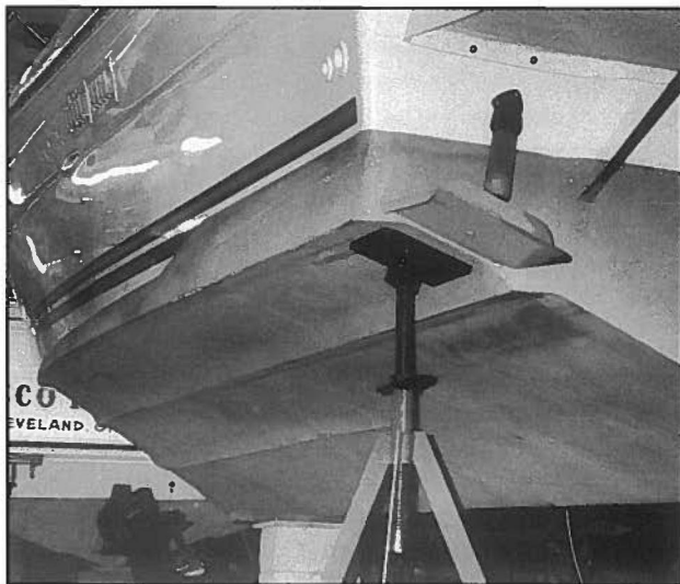
A chine—the sharp angle at which the sides of a boat's hull meet the bottom—provides this deep-V powerboat with better control and a dry ride at planing speeds.
