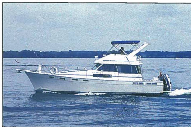
A power cruiser's flying bridge, usually called a flybridge, is an upper steering position originally intended as a platform to spot game fish.
